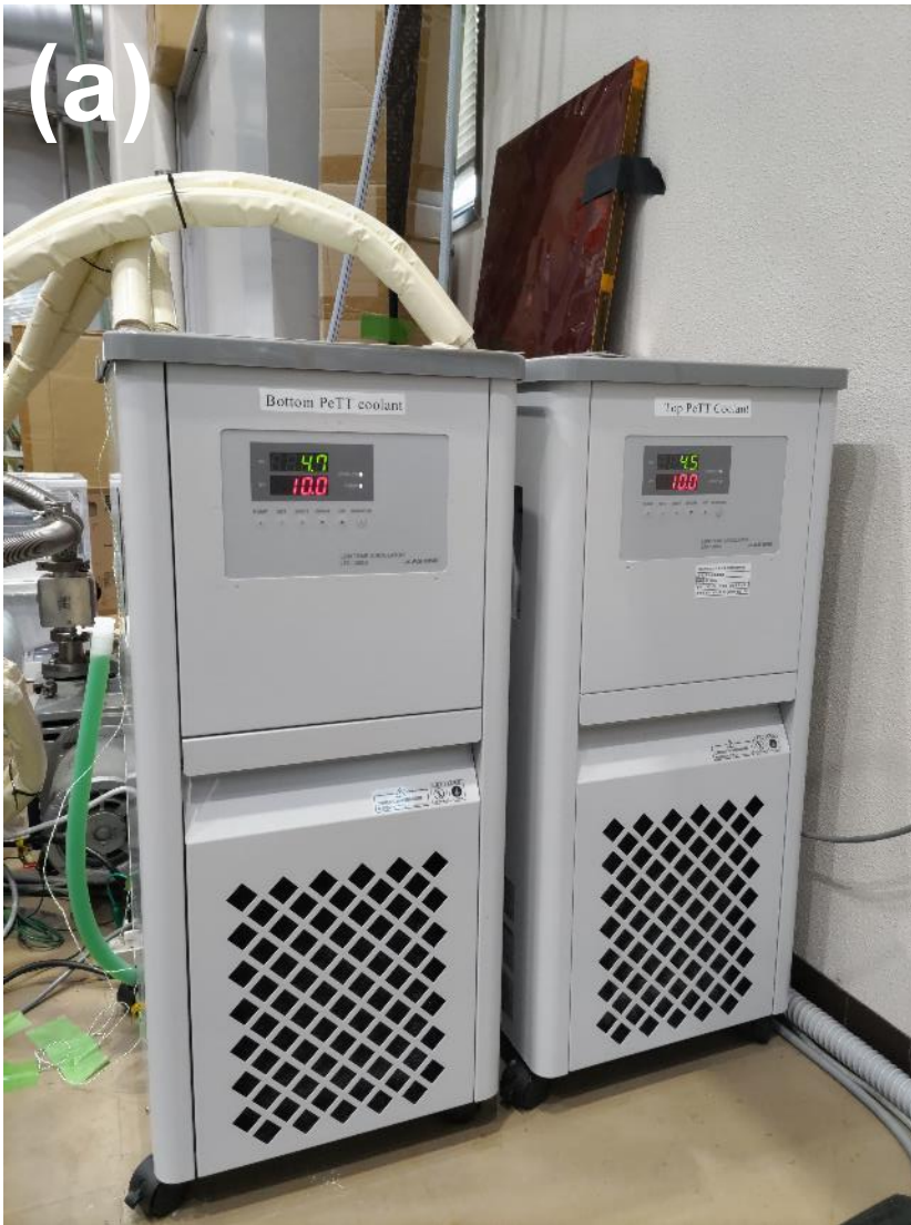
Fig. 4 (a) Coolant circulator station,
