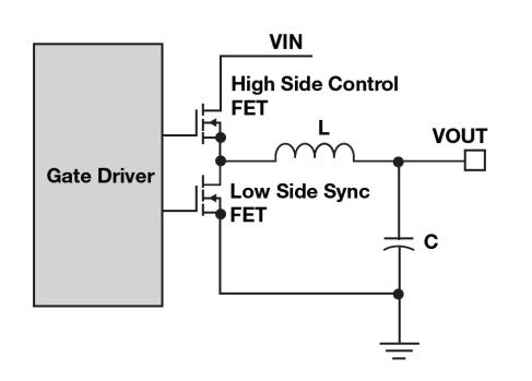
"is a circuit that uses power switches and energy storage devices to transfer energy from input to output. They can stepup, step-down, and invert"
